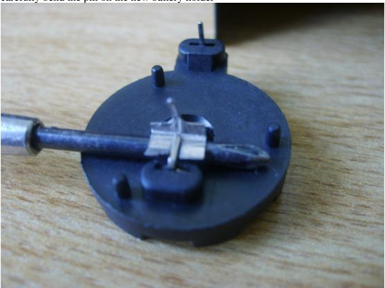
Now use a precision screwdriver to hold the tab, as shown in the photo below
