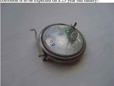
the photo below shows the battery removed from the board
