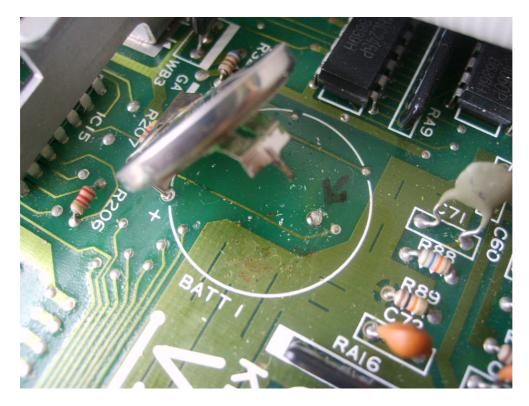
This picture shows the old battery removed from the board. This battery was completely dead, and the DDD1 lost all its settings and patterns from memory when switched off, causing a system reset every time it was switched on.
